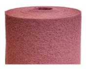
118 is an open structure aluminium oxide non-woven nylon fibre. It is used for light deburring and satinizing of metals with a low stock removal. Water and oil resistant.
